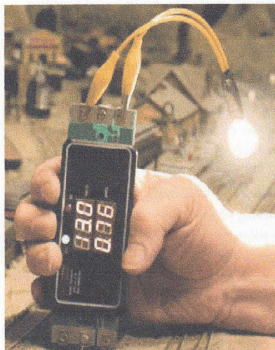
Checking voltage drop with an RRampMeter. Auto lamp used as a load.
